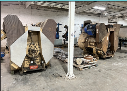
(2) Pioneer Pellet Mill each with (2) 200 HP Motors
