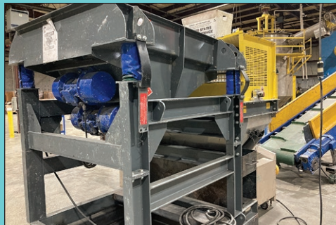
Paramount II Model FRC30-17 32" x 14" Vibratory Screener
