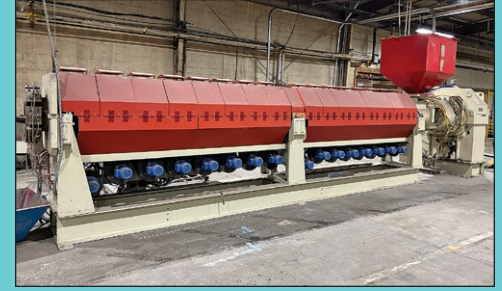
10" Mitsubishi Model ME250-3 Single Screw Non Vented; 600 HP Motor
