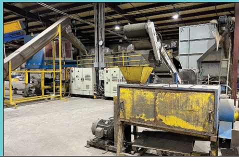
Shredding Line w/Separators, Sink, Float, and Dryer
