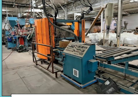
6" Johnson Extruder with 3.5" Johnson Co Extruder w/ 64" Wide Crown Sheet Line
