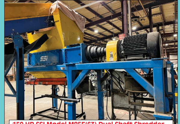
150 HP SSI Model M85E(63) Dual Shaft Shredder (New Gear Box)
